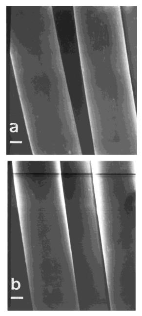
**Figure 3** Micrographs of (a) ungrafted and (b) 8.6% ethyl acrylate–grafted PET fibers (bar = 0.1 mm).
